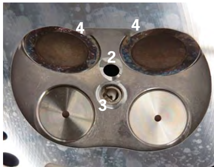
Injector position and combustion chamber design 2_10_17
