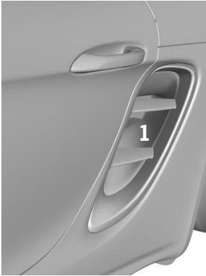
Left air intake
