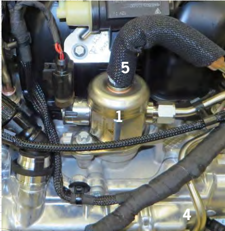
Fuel high-pressure pump (DFI) 2_07_17
