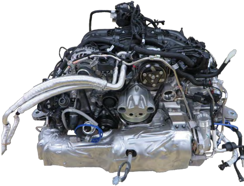
2.0 l 4-cylinder turbo engine 718 Boxster MY17
