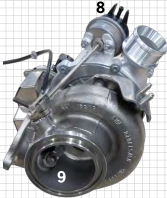
VTG turbocharger in 718 Boxster S MY17 2_36_17
