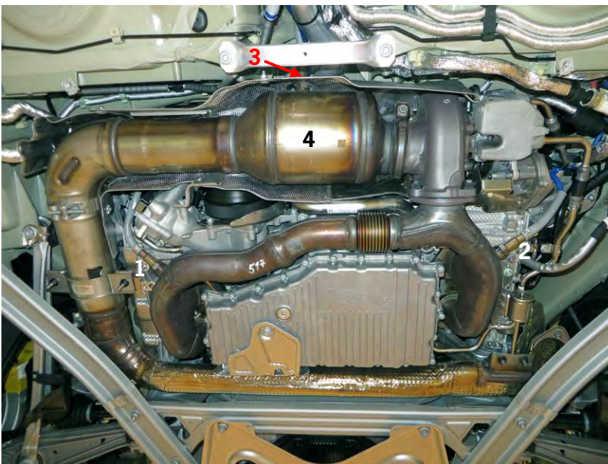
Installation positions of oxygen sensors
