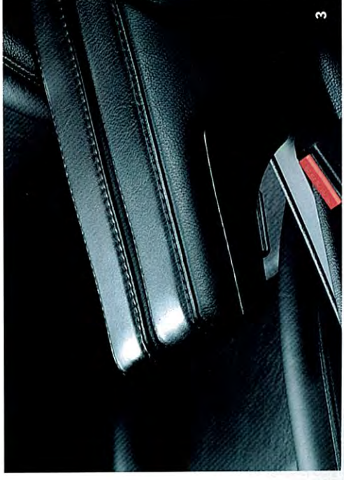
Armrests 911 (type 993 & 964) Leather-covered armrests with decorative double seam for retro-active fitting to seat backs. The armrests can be folded up separately and separately adjusted to any angle (Fig. 3).
