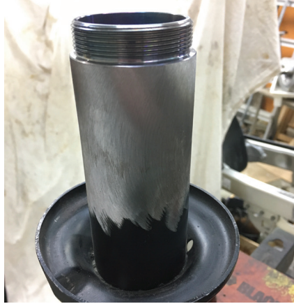
16 Once we confirm the height is right it is time to take the strut body to your local welder. TIG welding of the collar to the strut body should be around $30-$40 per strut and it should come back looking like this.
