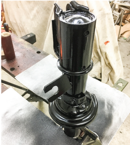
17 Sand down with 180 and 320 wet and dry and it is time to primer and paint.
