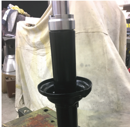
18 And then it is simply a matter of putting in the Bilstein insert, greasing the gland and tightening the top cap down to 130 +/- 10 Nm
