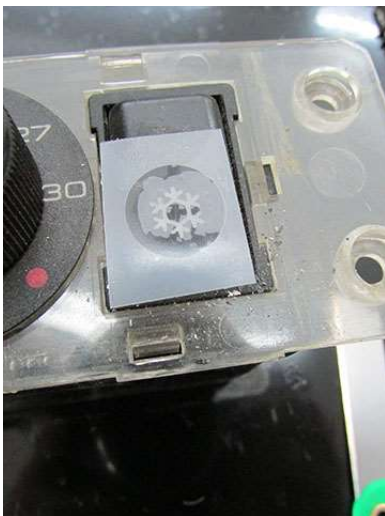
5d Apply the graphic making sure all of it is transferred.
